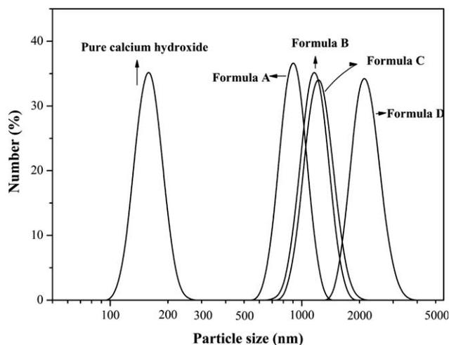
FIGURE 2. Particle size distributions of calcium hydroxide and microcapsules.
