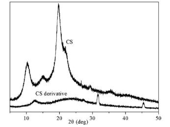
Figure 3 XRD patterns of the CS and thiolated CS derivative.
