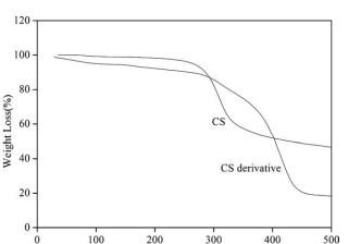
**Figure 4** TG curves of the CS and thiolated CS derivative.
