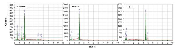
Fig. 4 Surface composition of NANOZR, 3Y-TZP and CpTi.
