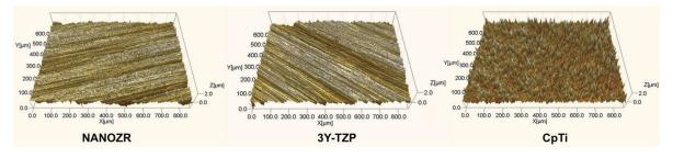
$Fig.~1~~3D~surface~topography~of~NANOZR,~3Y-TZP~and~CpTi~(0.6~mm \times 0.8~mm)~after~polishing~with~600 \#~abrasive~paper.$
