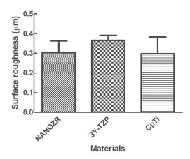
Fig. 2 Surface roughness of NANOZR, 3Y-TZP and CpTi after polishing with 600# abrasive paper.
