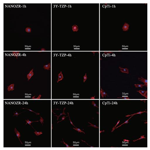
Fig. 8 Observation of actin cytoskeleton and cell nucleus of MC3T3-E1 on NANOZR, 3Y-TZP and CpTi after 1 h, 4 h and 24 h incubation.
