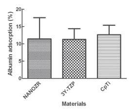
Fig. 6 Bovine serum albumin adsorption rates of NANOZR, 3Y-TZP and CpTi after 1 h incubation. There was no significant difference among the three materials (p>0.05).
