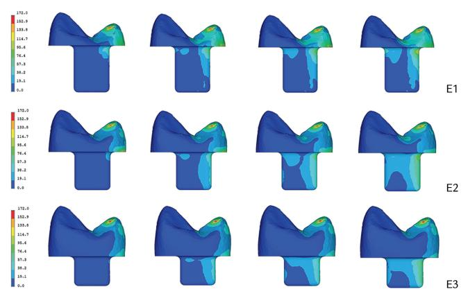
Figure 6. Von Mises stress distributions (MPa) in models E1, E2, and E3 in endocrown under oblique load of 200 N.
