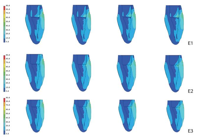
Figure 7. Von Mises stress distributions (MPa) in models E1, E2, and E3 in dentin under oblique load of 200 N.
