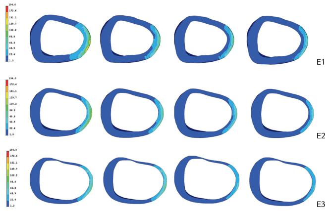
Figure 5. Von Mises stress distributions (MPa) in models E1, E2, and E3 in enamel under oblique load of 200 N.
