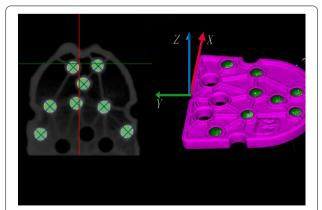
**Fig. 5** Coordinate alignment in the implant planning software. Left: The software identified the zirconia beads in the diagnostic plate in the image. Right: The positions of the diagnostic plate and the radiographic template were aligned with the coordinates of the software
