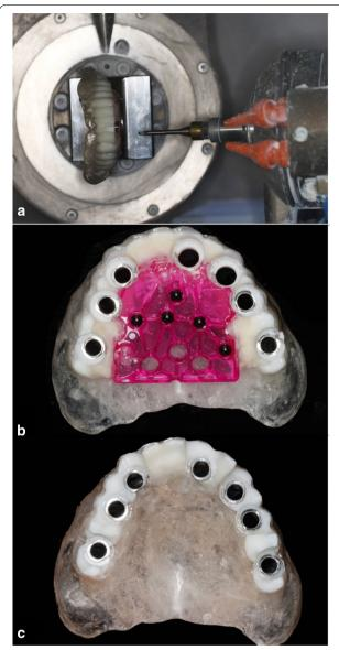
**Fig. 6** The radiographic template was transferred into the surgical guide by the CNC milling process. **a** The radiographic template was fixed on the holder of the CNC milling machine, and slots of the sleeves were milled on the radiographic template. **b** Steel guide sleeves were installed into the slots. **c** The registration template was removed, and the radiographic template was transferred into a surgical guide
