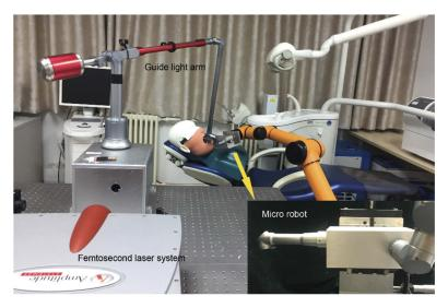
Fig. 1. Photograph of the automatic tooth preparation robot.
