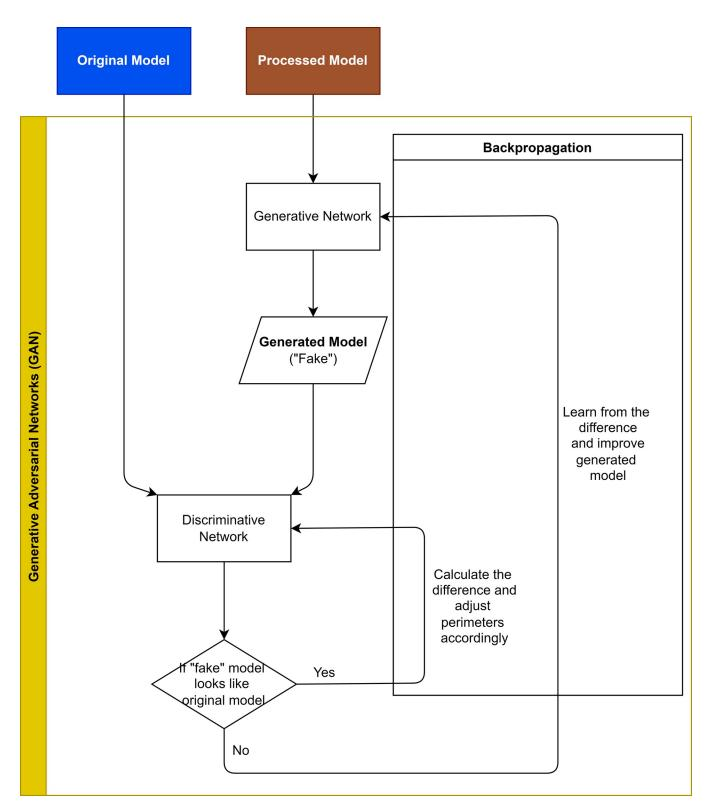
Fig 3. Brief architecture of the Generative Adversarial Network (GAN) of this study. Original model: digitized maxillary teeth model collected from participants; processed model: teeth model with tooth 16 removed; Generated model: teeth model with AI-generated tooth 16.
