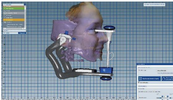
Fig. 8 CBCT scan, face scan, bite fork scan and dental arch scans uploaded into the Virtual Artex CR digital articulator (Amann Girrbach, Germany)
