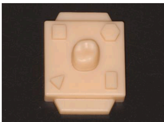
Fig. 2. Three-dimensional analysis model of computerized numerical control-cut zirconia crown abutment.
