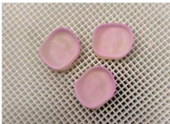
Fig. 3. Nano-silica–lithium coating on the internal surface of zirconia crowns.
